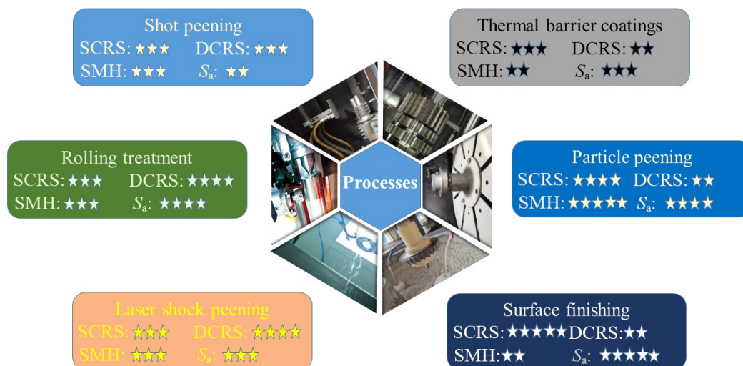
Fig. 21 Gear surface manufacturing processes (number of stars represents potential to improve surface integrity).
