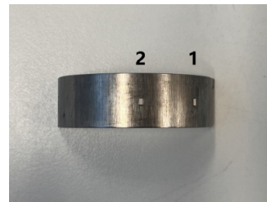
Fig. 7 Undamaged aluminium alloy-coated bearing shell and layout of sensors for ultrasound frequency tests.
