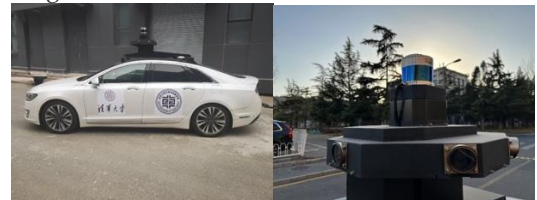
Fig.4 Test vehicle and its sensor configuration
