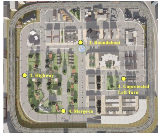
Fig. 3 Test scenarios in CARLA Town03. For each location, background vehicles are randomly initialized in number and state, while following rule-based driving policies with location-specific, fixed behavior parameters, resulting in distinct yet consistent interaction patterns across locations.
