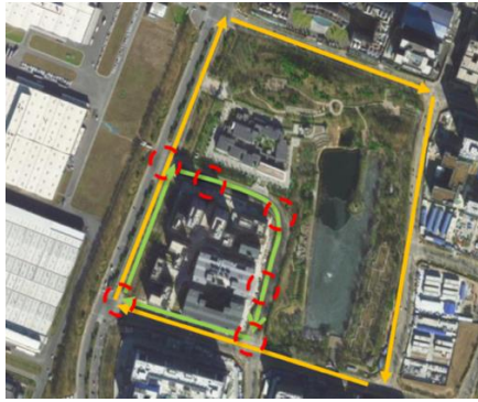
Fig.5 Real-world test route in an urban industrial area. The inner loop (shown in green) is a 1.0-km circuit covering intersections, an industrial-park entrance, and roadside parking zones, while the outer loop (shown in yellow) extends the route to 2.1 km by including major merging segments and arterial roads.
