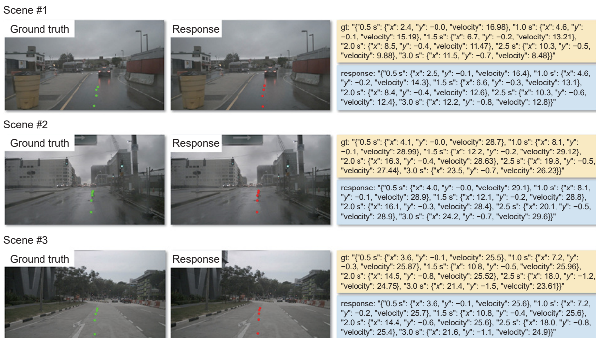
Fig. 6 Long-tail successes. Green denotes the ground truth trajectory, and red denotes the model response. Some trajectory way-points cannot be fully shown in the front-view image due to field-of-view limits. The Top-K value of RAG is set to 2 accordingly. The VLM backbone is Qwen2-VL-2B.
