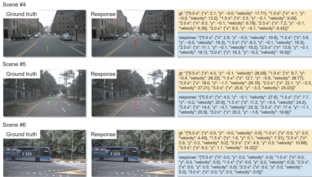
Fig. 7 Failure case analysis. Green denotes the ground truth trajectory, and red denotes the model response. Some trajectory way-points cannot be fully shown in the front-view image due to field-of-view limits. The Top-K value of RAG is set to 2 accordingly. The VLM backbone is Qwen2-VL-2B.
