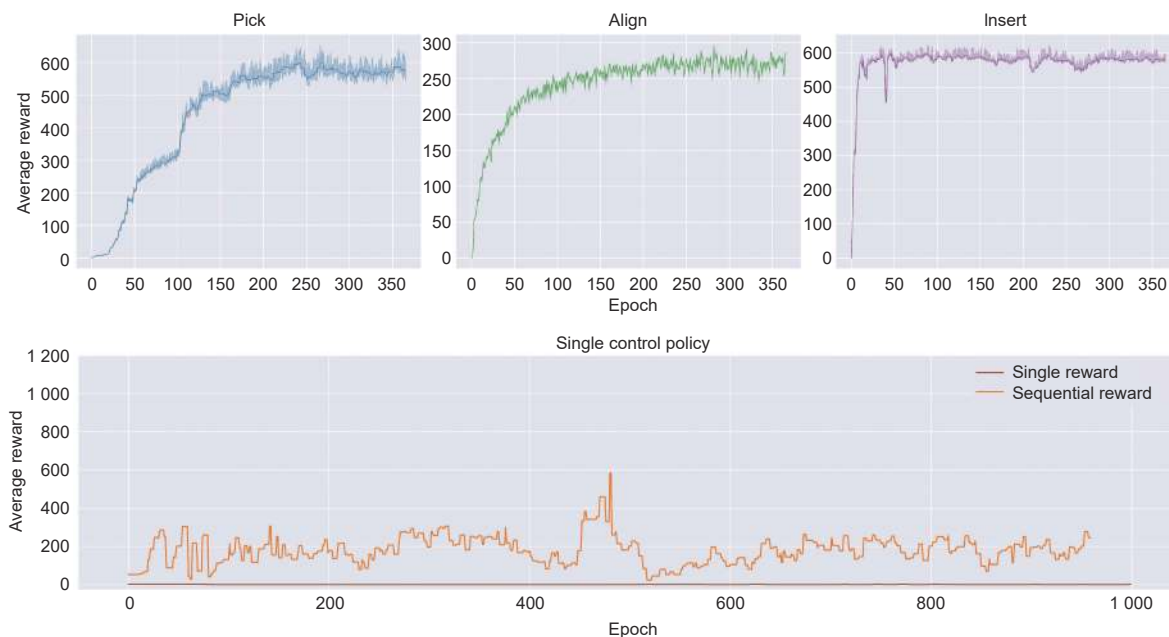
Fig. 7 Policy learning curve for sequential control policy (top) and single control policy (bottom). The top three plots represent the average reward curve in each training epoch of control policies for three sub-tasks. The bottom plot represents the best training process of a single control policy with two reward functions within the same epochs.
