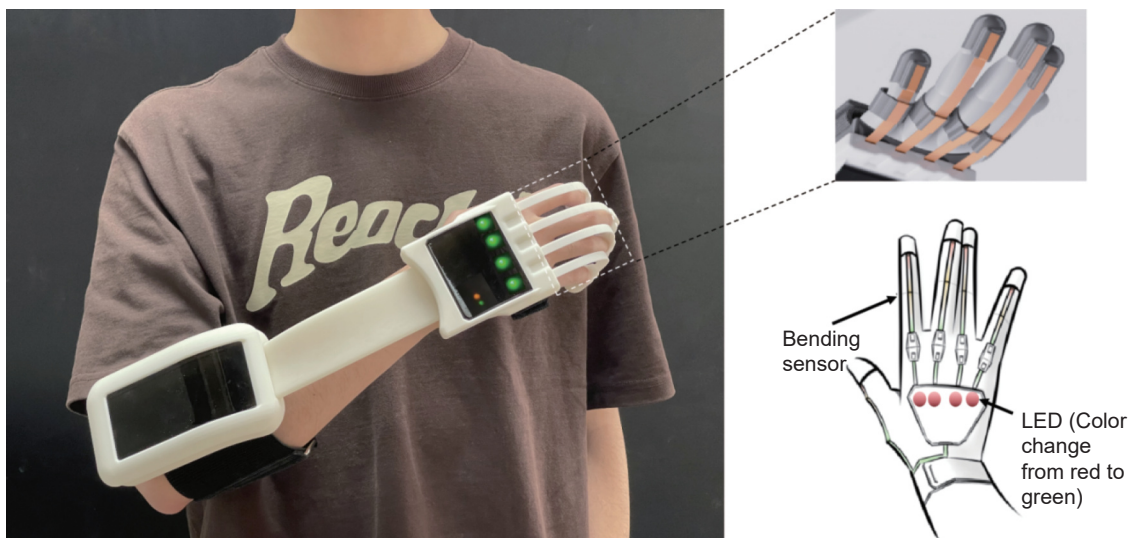
Fig. 2 The fabricated hand rehabilitation product integrated with curvature sensors and visual feedback element (LED).
